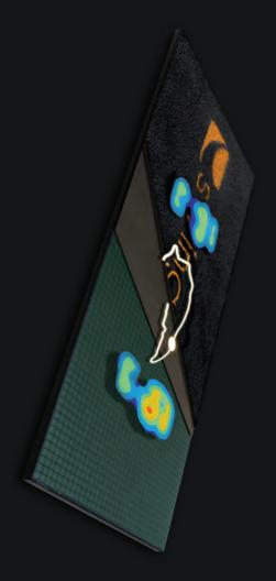
Real-time data is perfectly synchronized with high-speed video images and displayed on-screen. This makes it possible for you to see exactly how and when you transfer weight and distribute foot pressure during a golf swing.
